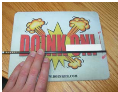
A mouse pad provides an ideal flat surface for marking where to apply the vinyl
